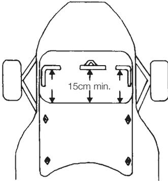
Lower end of bubbleshield showing minimum 15cm gap between shield and pedals. Also indicating the maximum 4 fixing points if shield attached to bodywork.
