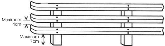
If open type fencing or railing is employed, the gap at the bottom should not be more than 7cm in height, and the gap between the rails not more than 4cm. The support posts must not protrude above the level of the top rail.
